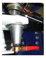
Click OK to make the Z-axis move down and touch off the inverted tool holder and then raise up to a safe distance and move back towards Y=0.
