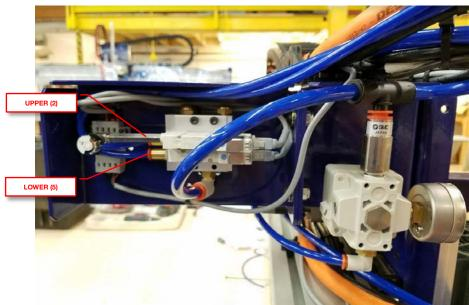
Turn on the pneumatics switch at the filter regulator manifold and verify that the pressure here is between 90 and 100 psi.
