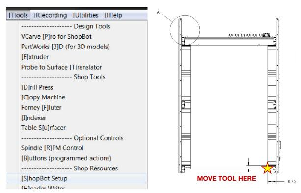
Go step-by-step through this window while verifying information about the machine. Make sure that the check boxes for the Z zero plate and proximity switches are checked at the bottom of the window. Select the radio button marked ATC4. (If your ATC tool has a pneumatically actuated dust foot please call ShopBot for support and an alternate document).
