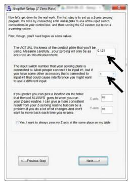
In the "ShopBot Setup (Z Zero Plate)" screen, measure the thickness of the plate and enter that value. Make sure the input switch is set to "1". DO NOT check the "Yes, I want to always zero my Z axis at the same place on my table". Click "Next"
