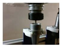
**Note:** This should only be a move in the Z-axis so that the tip of the drill rod is below the top edge of inverted clip. Do not move X or Y axes.
