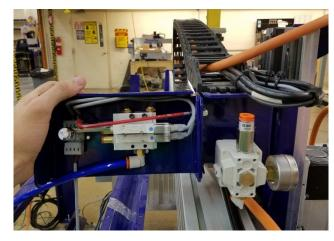
Using a 4mm hex wrench and adjustable wrench, connect the ATC manifold to the Y-Echain Bracket on the rear of the YZ car using the pair of pre-mounted hardware as shown above.
