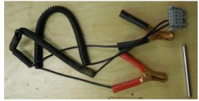
The red calibration clip will be clipped to the bottom of an empty tool holder as it is moved through all of the clip positions.
