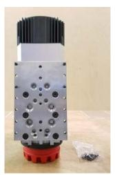
The ShopBot ATC is equipped with a 5HP fan cooled HSD spindle. An ATC system requires a minimum of 7 scfm at 100 psi of clean, dry, un-oiled compressed air which will be internally regulated to the following pressures:
