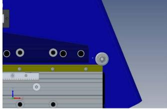
The Fixed Z-zero plate can now be wired directly into the control box using the attached 2 conductor cable. Connect the cable to the plate with the attached WAGO connector and wire the black and red wires into ground and input 1 (ZZ) respectively on the control board.
