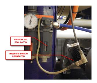
Inside the control box, route the pressure switch cable to the ATC interface board. Connect the blue two pin terminal block to the location marked "pressure switch."
