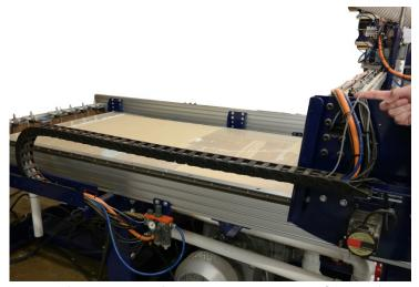
Run the ferruled side of the 3-conductor 30' ATC cable from the pneumatic manifold through the Y and X cable carriers and into the control box and to the ATC interface board as shown in the picture to the right.
