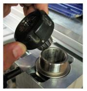
Install the bit in the collet and hand tighten the collet nut so that the bit does not slip down into the collet.
